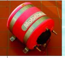
The Mobitherm has a capacity of 20 litres, and can be mounted horizontally and vertically. The water heater has simple feet spot-welded to a strap that goes round the tank. Both the tank and heat exchanger are made of high-quality acid-proof steel (AISI 316). The insulation is of polyurethane foam, but is not equipped with any protective casing.
