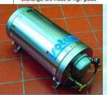
The Isotemp Slim 20 has a tank capacity of 20 litres. It can be mounted horizontally and vertically, but in that case with the connection points facing down. The water heater has strong feet that are spot-welded to a strap that goes round the tank. Mixer thermostat and heating element are standard.
