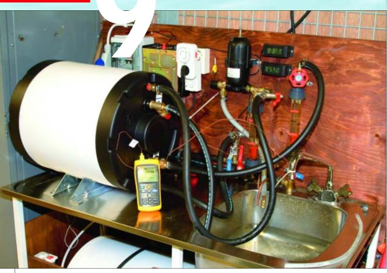
TO ENSURE THAT the test results were repeatable, and that the tanks operated in identical conditions, they were tested on the bench. Here the tank of the Vetus is connected.
