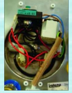
SAFETY THERMOSTAT: The Isotemp is the only water heater in the test with a safety thermostat that works on boiling dry. The blue "box" is the safety thermostat, while the operating thermostat is the white "box".
