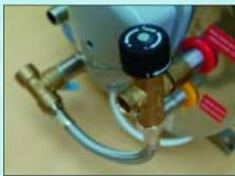
MIXER VALVE: The tanks from Isotemp have a mixer valve as standard. The temperature of the water to be supplied by the heater is set here. Cold water is mixed in with the hot water to attain the correct temperature.
