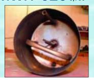
SIMPLE CONSTRUCTION, and the material is acid-proof AISI 316 steel. The test shows that the heat exchanger is rudimentary. The tank is identical to the QL.
