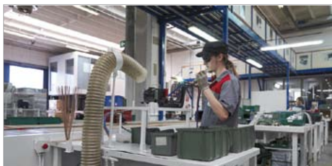
Welding of the condenser to the compressor
