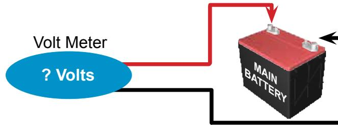
With the engine running, measure the voltage across the terminals of your main battery using a voltmeter. **The voltage should be above 13.7 volts.** Turn on the vehicle lights, air-conditioner and any other load (such as spot-lights). Measure the voltage on the battery again. If the voltage has dropped below 13.5 volts then it is recommended that the alternator performance be checked.
