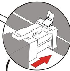
Plug one end of the cable into the port of the Intelligent Solenoid .
