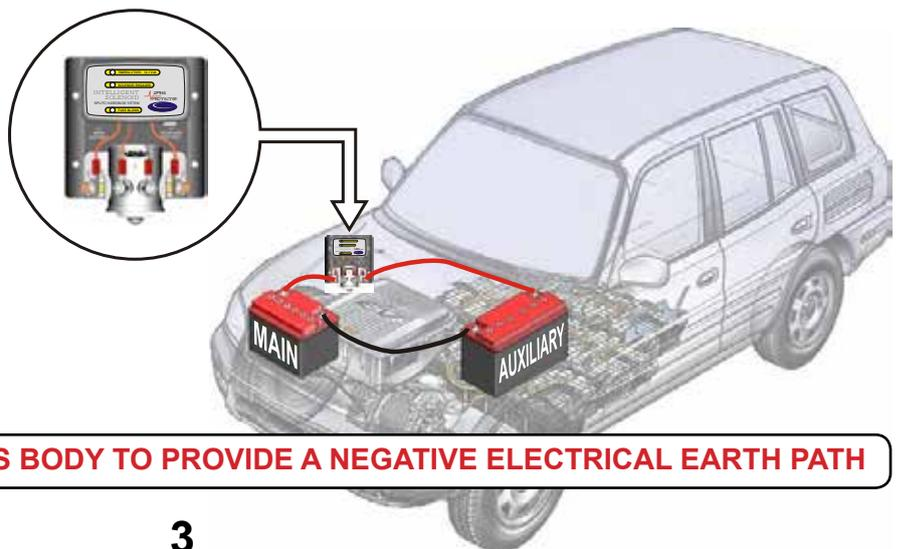
**DO NOT RELY ON THE VEHICLE'S BODY TO PROVIDE A NEGATIVE ELECTRICAL EARTH PATH**
